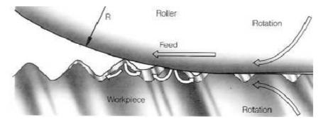
Figure 1: Basic Operation of Burnishing
