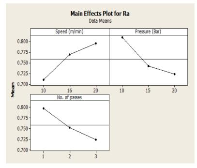
Figure 4: Effect of Control Factor on Surface Roughness
