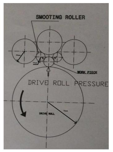
Figure 3: View of Multi Roller Burnishing Tool
